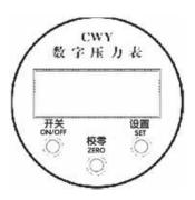
"Switch" key: turn on and off the machine. The instrument can be closed if we do not use; in doing so, power consumption can be reduced. Scanning this key, the starting point and the full measure range point of this instrument can be displayed within 2 seconds; the instrument is under measuring mode at this moment. Again, scanning this key for 2 seconds, the instrument comes into shutdown mode.
